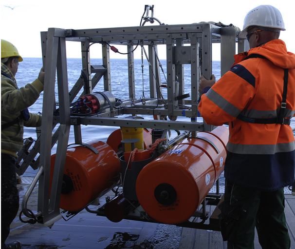
Figure 4. Photograph of Benthic Lander with HARP prior to deployment. Hydrophone is mounted horizontally above right-hand side orange tube toward the center of the lander, ADCP is yellow and pointing upward, and CTD is mounted horizontally to the frame (photograph by Peter Linke – GEOMAR). (For interpretation of the references to color in this figure legend, the reader is referred to the web version of this article.)
