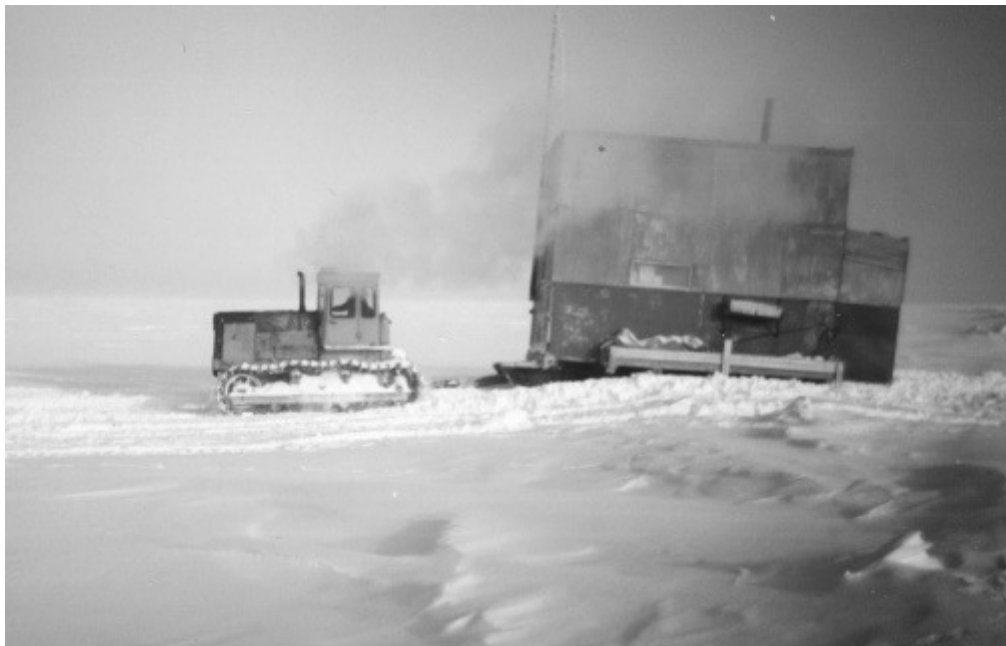
Figure 4.7-2: The caterpillar tractor S-130 and habitable mobile-home "balok" on the Laptev Sea ice.
