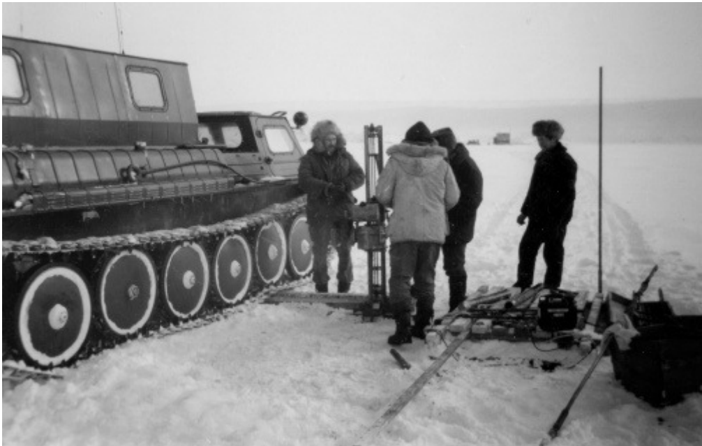
Figure 4.7-1: Drilling process with the drilling machine UKB-12/25 on sea ice.
