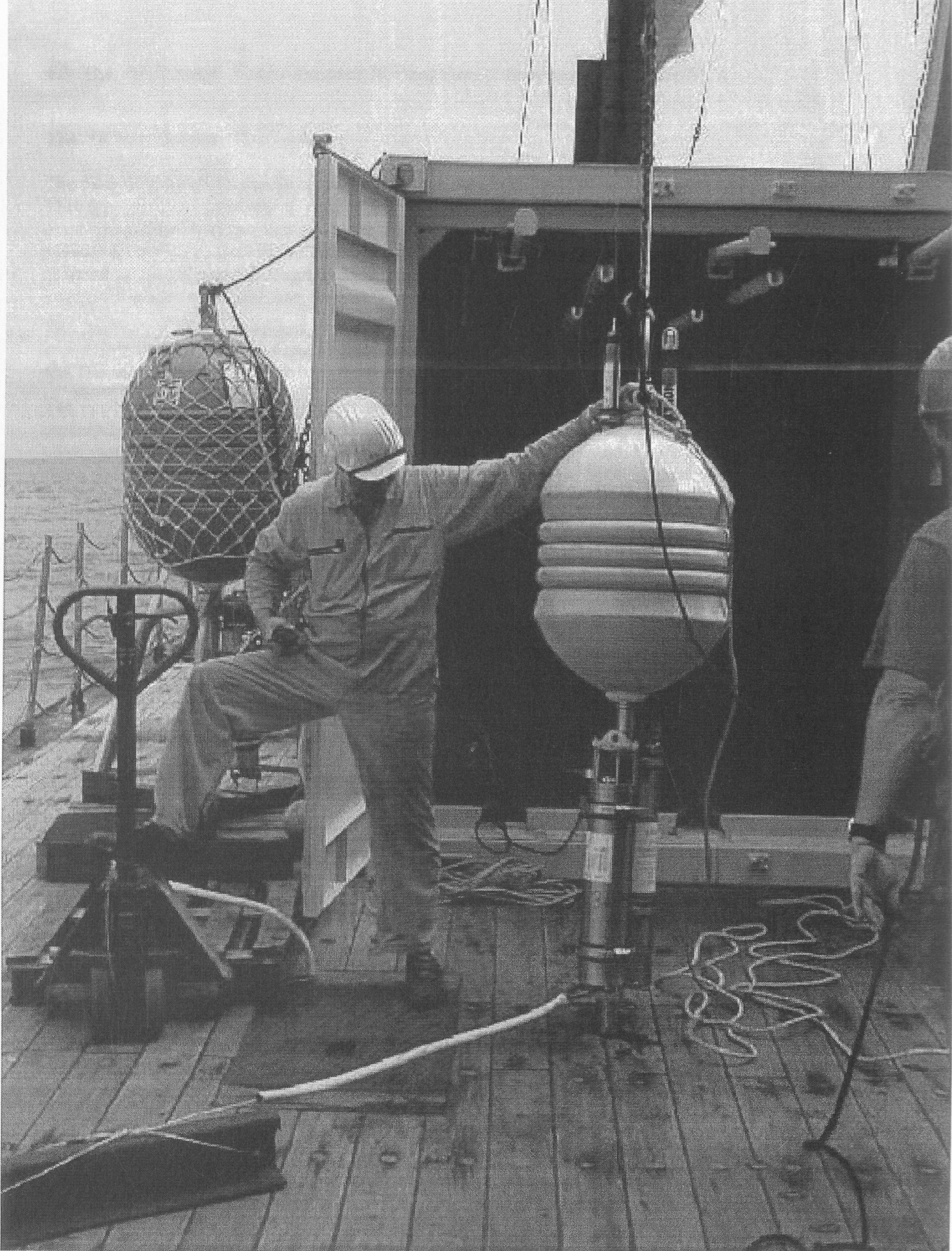
Figure 4.3.2: The GEOMAR OBH ready for deployment Background left: GEOMAR OBS Background right: OBH container
