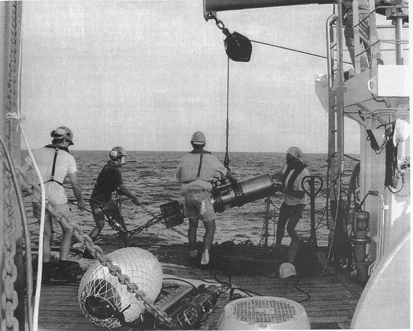
Figure 4.10.3 The array of Trakia Airguns. One of the airguns is shown during deployment operation.
