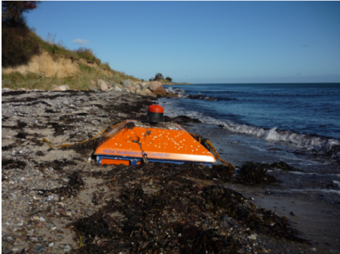
Figure 4.1: The buoyancy part of the mooring stranded off Langeland, DK, October 2011.
