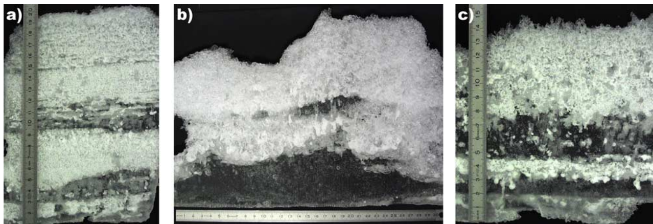
Figure 13. Photographs of vertical thick sections from surface cores comprising metamorphic snow, ice layers, and superimposed ice: (a) 30 December, FY1, (b) 20 December, SY2, and (c) 30 December, FY1. All scales are in centimeters. Note slightly different scales in Figures 13a–13c.
