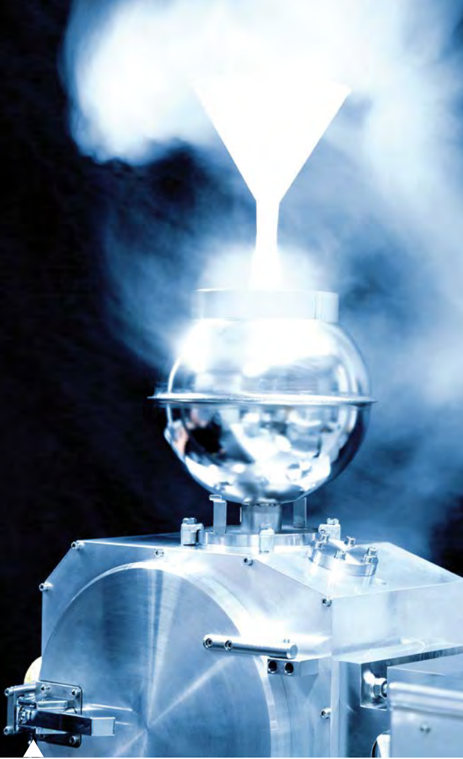
Cold trap at the thermal ionization mass spectrometer "TRITON" being filled with liquid nitrogen. Image: Pohl/Warnk/Gall
