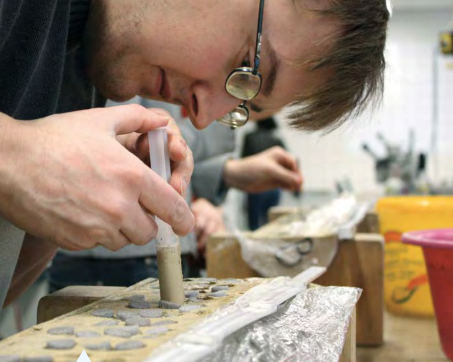
The seabed's climate archive: Sediment cores are vertical sections into the seabed that provide a record of the past. Precise analyses of their chemical composition yield critical data on the climate of the past. Image: Katja Machill, GEOMAR
