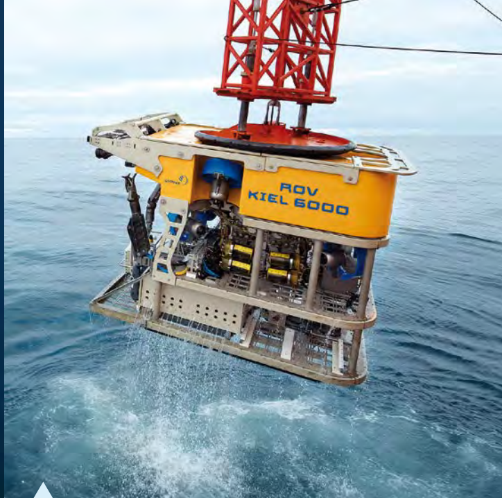
Eyes and arms in the deep sea: Remotely controlled deep sea robots, such as the ROV KIEL 6000, enable thorough exploration and testing of mineral deposits, for instance at volcanic-associated hydrothermal systems. Image: Bernd Grundmann
