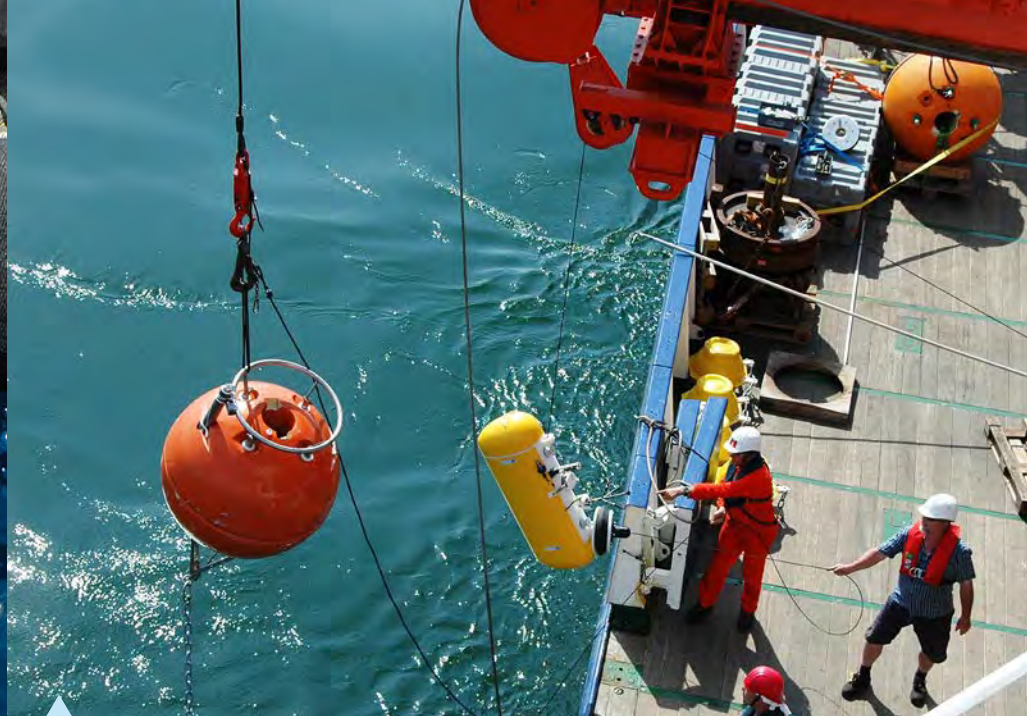
Deep-sea moorings: Measuring instruments are deployed at different depths to record various physical and chemical parameters for extended periods. Vertically installed measurement chains [moorings] allow long-term measurements at critical points in the oceans. Image: Michael Schneider, METEOR
