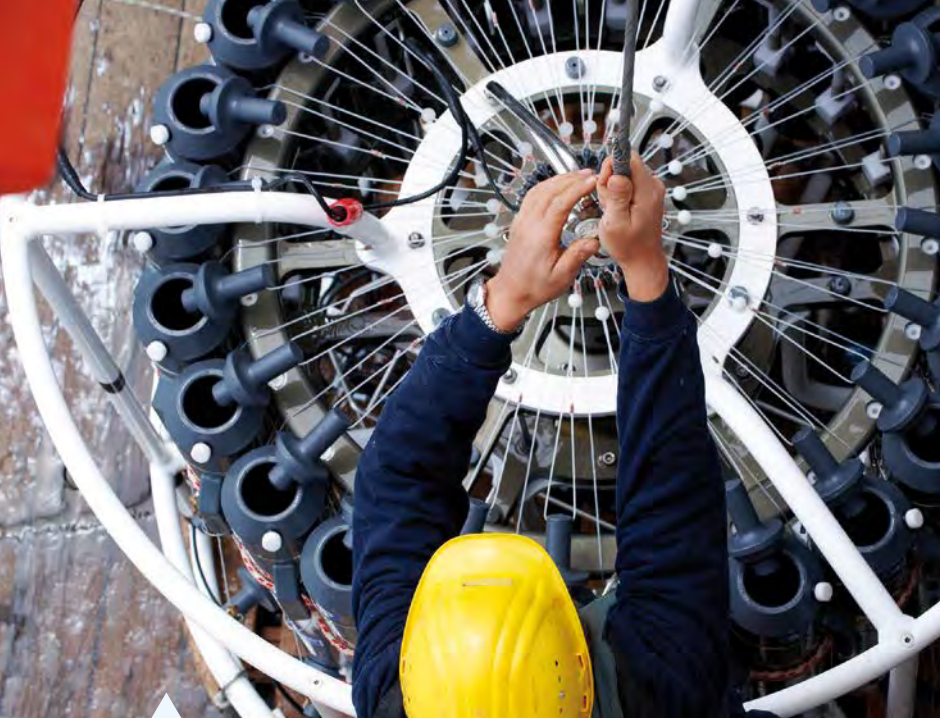
A rosette water sampler (CTD-Rosette) collects water samples from different depths. Valuable physical, chemical and biological data for a variety of questions concerning marine research are obtained from these deployments. Image: Bernd Grundmann
