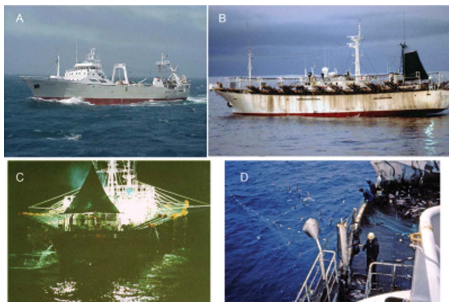
Figure 1. Vessels for squid fishing: (A) factory trawler; (B) large oceanic jigger; (C) jigger light fishing at night; and (D) drift netter.
