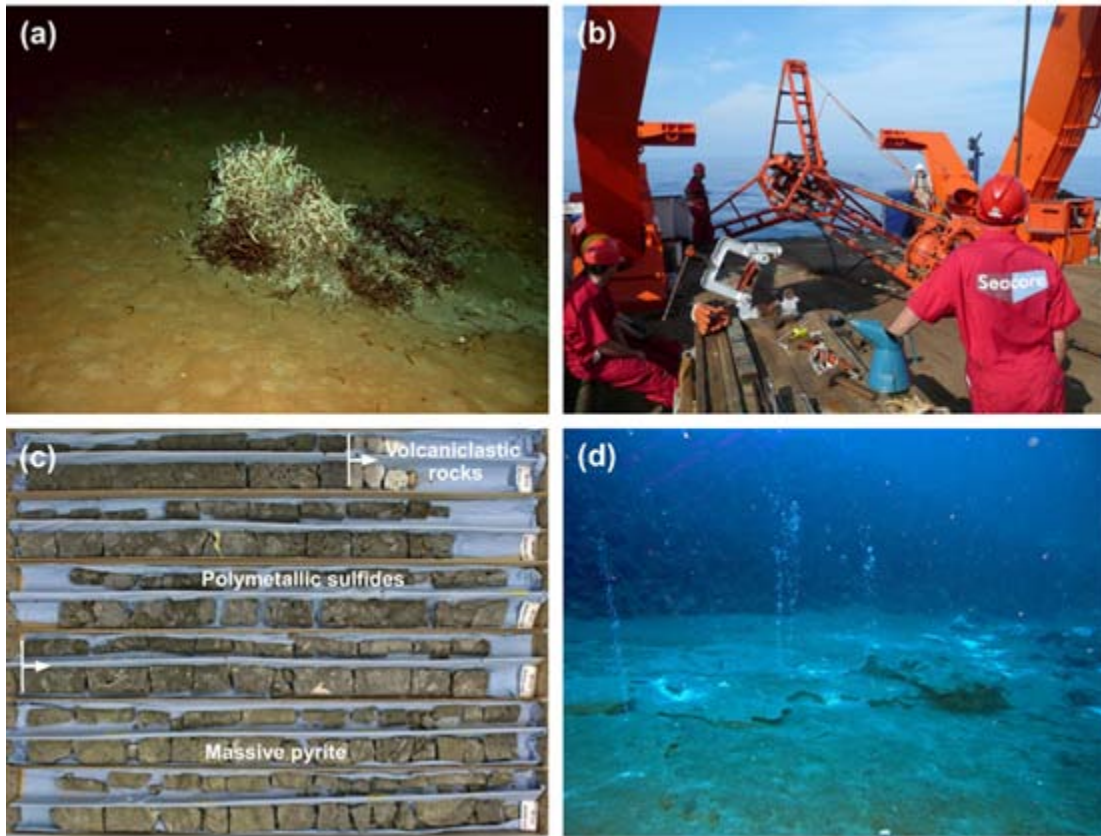
Fig. S2. (a) Seafloor image of a tube worm colony at Palinuro. Sediment covering the surrounding seafloor shows noticeable discoloration. (b) Operation of BGS Rockdrill on board R/V Meteor. The lander-type drilling device permits drilling to a depth of 5 meters below seafloor. (c) Representative drill core of massive sulfides from Palinuro. Altered volcaniclastic rocks are underlain by polymetallic sulfides. The lower part of the core consists of massive pyrite (hole 865RD; top of core to the right; width of core box is 1.0 meter). The mineralization is locally crosscut by native sulfur veins. (d) Seafloor image of a hydrothermal explosion crater at Panarea. Sediments surrounding gas vents are indurated and partially cemented by native sulfur. A low-relief wall surrounding the crater can be observed in the background.
