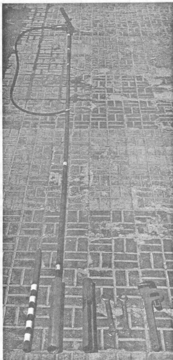
Figure 4.1 Pneumatic drill with extensions, drill bit and core catcher. Photograph: John J.G. Reijmer.
