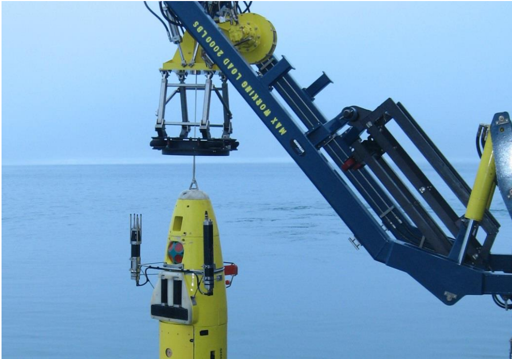
AUV Abyss (autonomous underwater vehicle).
