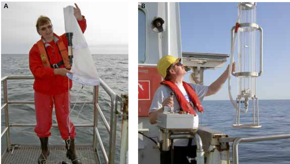
Figure 2.10 Sampling of water for analysis of phytoplankton (panel A) and chlorophyll-a (panel B) of an algal bloom.
