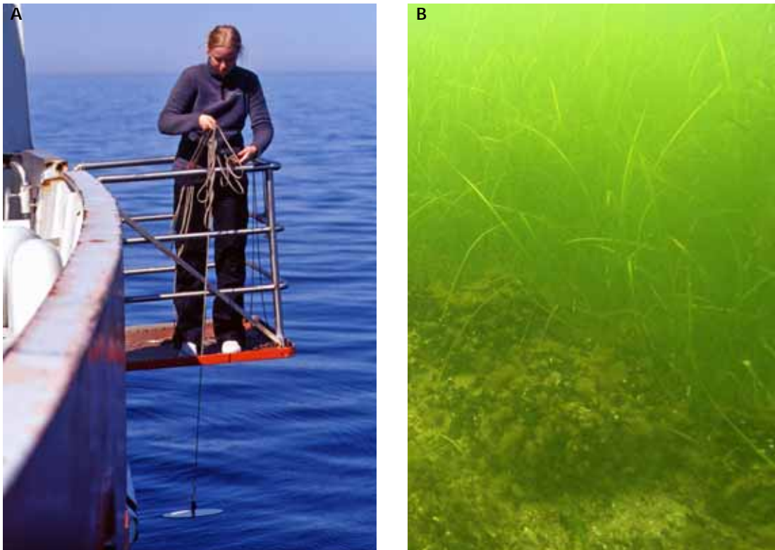
Figure 2.16 Secchi disk used for measurements of water transparency (panel A) and low water transparency (panel B).
