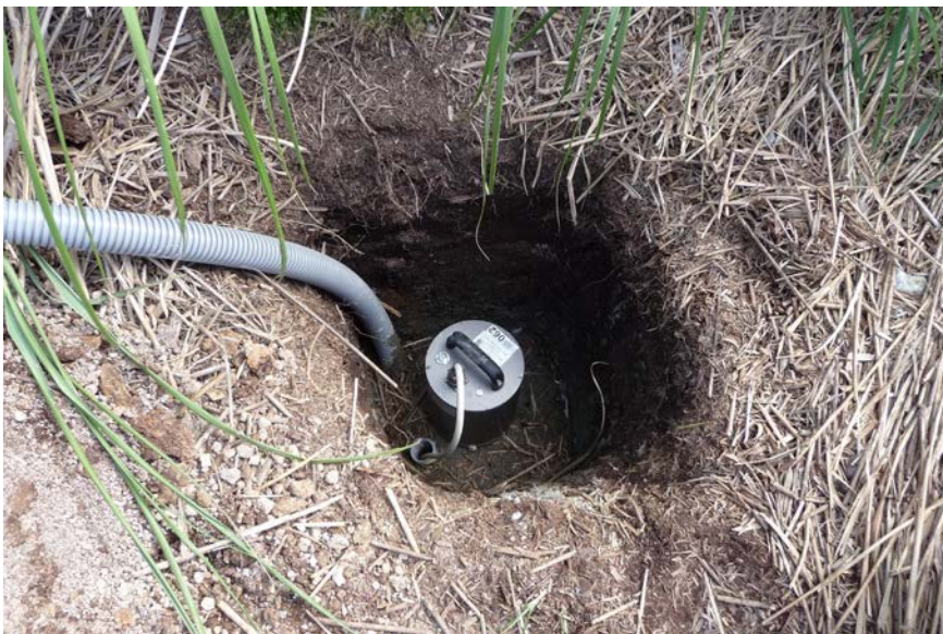
Fig. 5.3.3 Preparation of seismometer basement at site NIG01.
