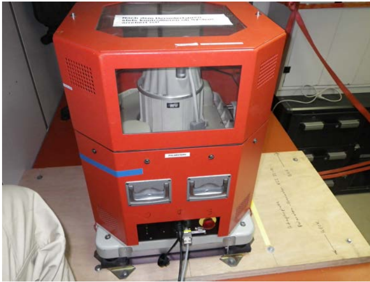
Fig. 5.4.4 Installation of the sea gravimeter in the gravimeter room. View in direction towards bow.
