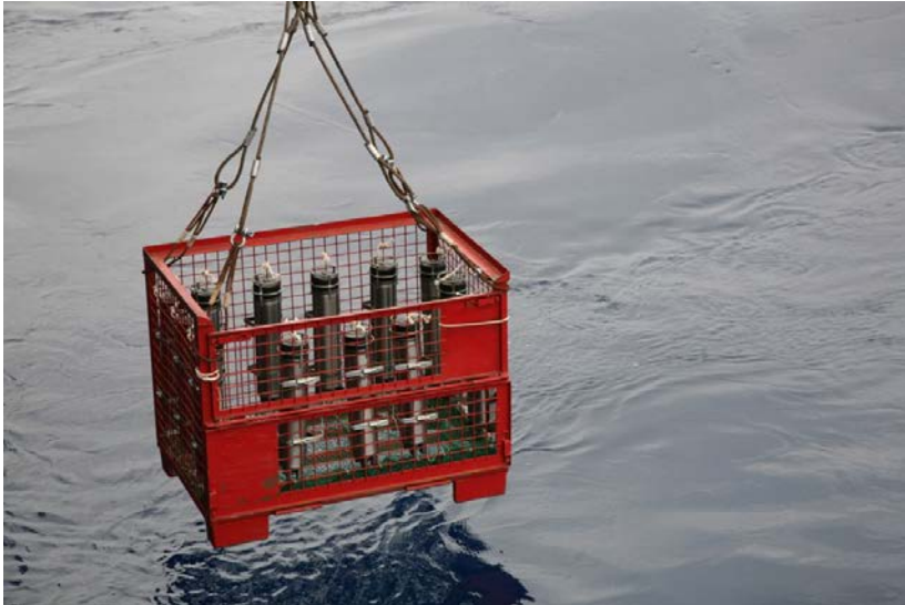
Fig. 5.3.2 Photograph of the releaser test configuration (Photograph by M. Retief).
