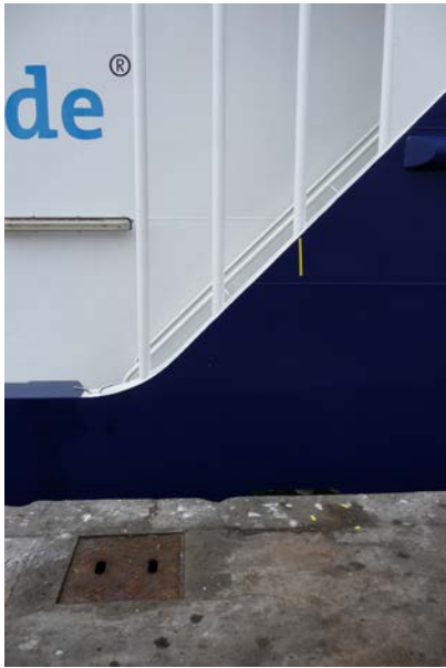
Fig. 5.4.1 Tie measurement site at the pier in Walvis Bay. The yellow stripe at the ship marks the horizontal position of the gravimeter inside the ship.
