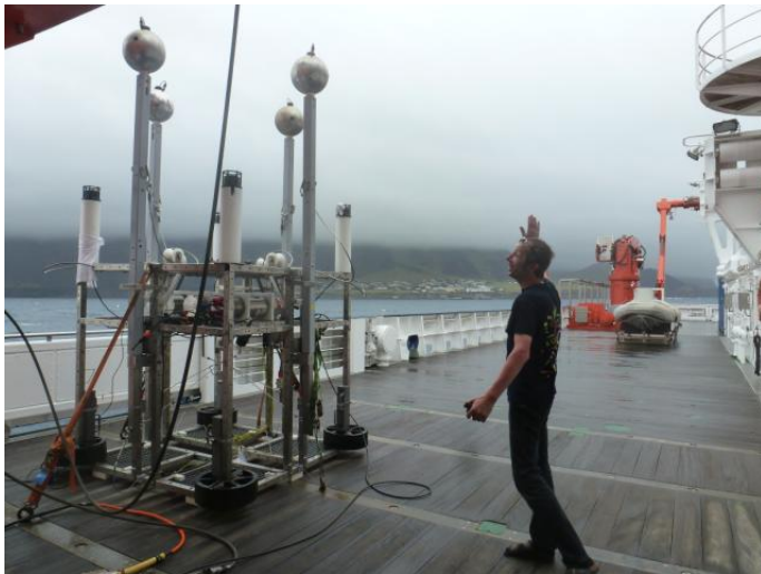
Fig. 4.5 Newly developed electromagnetic Sputnik transmitter which was undergoing last testing at the Mid-Atlantic Ridge.
