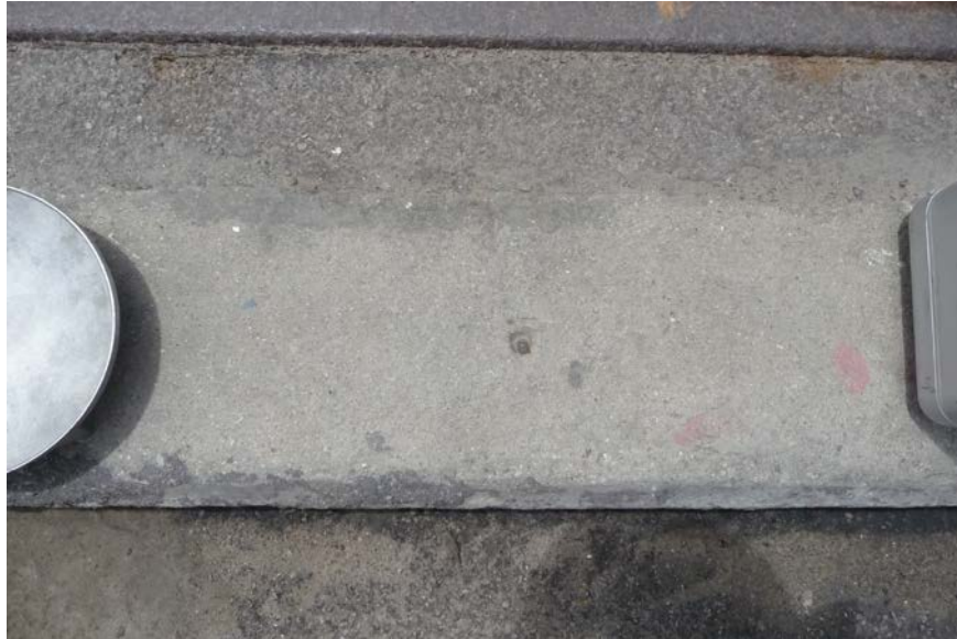
Fig. 5.4.3 Gravity tie point WALVIS-W17. Note the marking nail in the centre.
