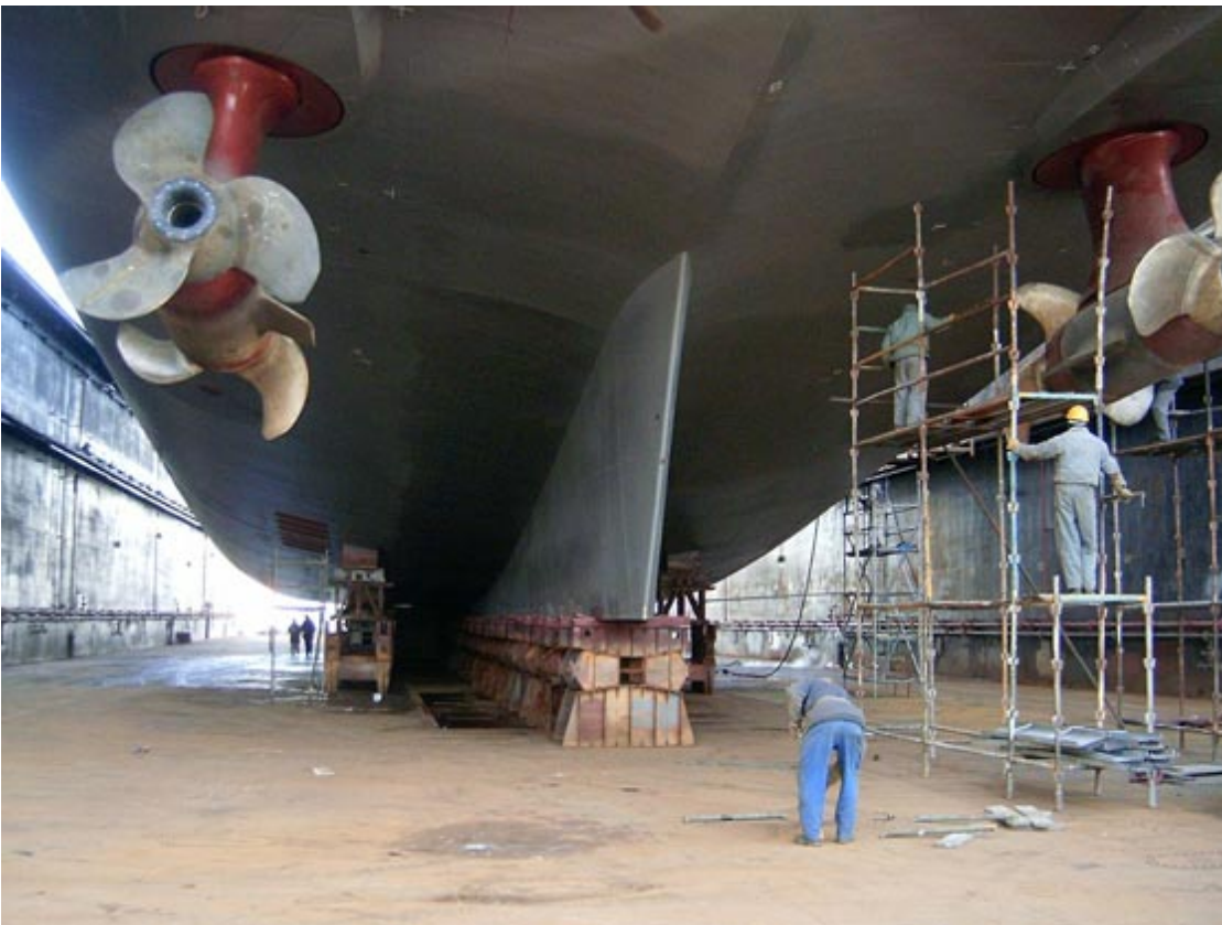
RV MARIA S. MERIAN in a dry dock showing its special propulsion systems. Photo: Achim Schüler
