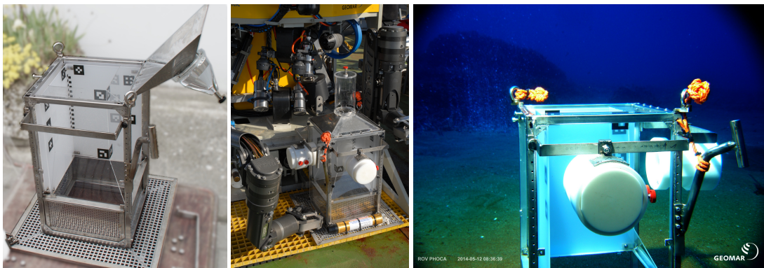
Figure 2. Three views of the bubble box, from left to right: box without cameras during development, box on ROV Phoca before being deployed (research cruise on RV Poseidon) and box in shallow water near Panarea, an area with heavy carbon dioxide release.
