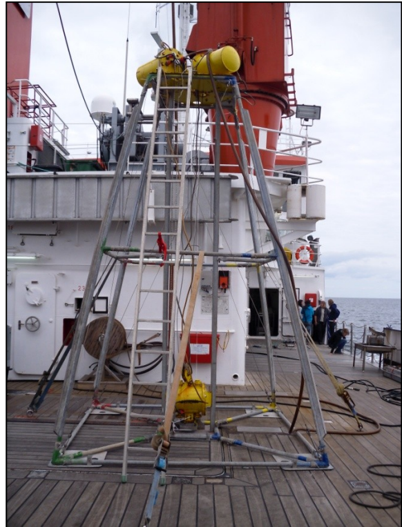
Fig. 8: Lift Tower with VK200 Vibro Coring System aboard R/V Alkor (Photo: Joost Thielsen)
