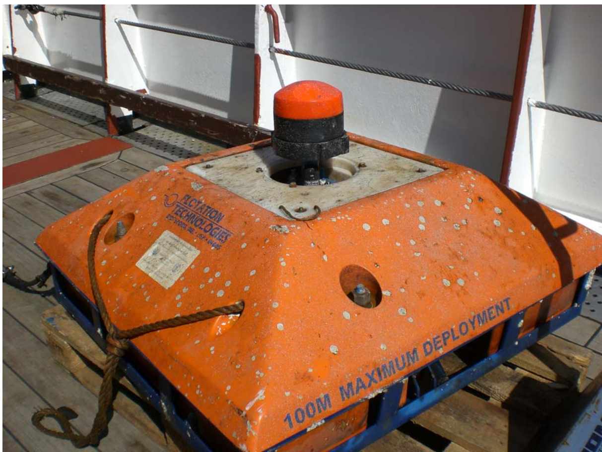
Fig. 5.1: the trawl resistant bottom mooring's flotation part after 9 months deployment in mooring V431-18. On top the RDCP's transducers. The MicroCat is attached to the weight (not shown here). The total weight is about 1.500 kg.
