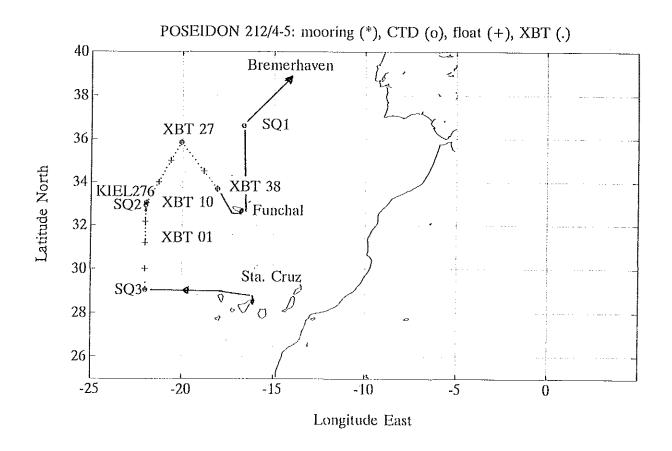
Poseidon cruise 212/4-5, 10. - 29.10.1995, Sta. Cruz - Funchal - Bremerhaven: Mooring KIEL276 exchanged, moorings with sound sources are SQ1/V368, SQ2/V369, and SQ3/V370. Positions of launched floats and XBT drops are indicated.
