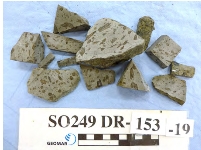
A highly hornblende-phyric spessartite, a typical rock of the Komandorsky Block dredged in ~2,100 m water depth at its northern tip. The huge hornblende crystals are clearly visible under a microscope (small picture). (photos: GEOMAR)
