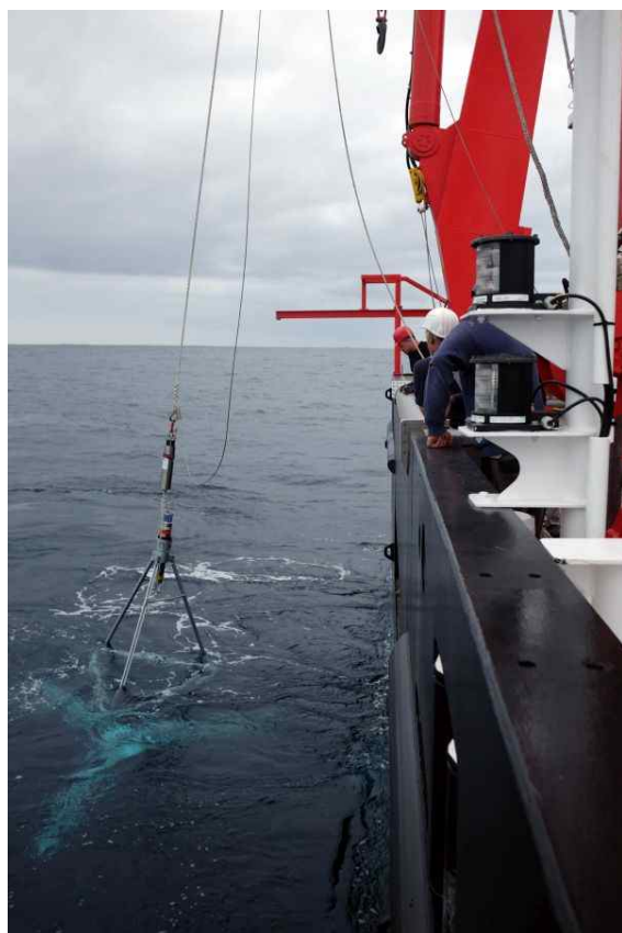
Figure 6.1.2.4: The tripod on the deep-sea cable above and below the water (J. Steffen).
