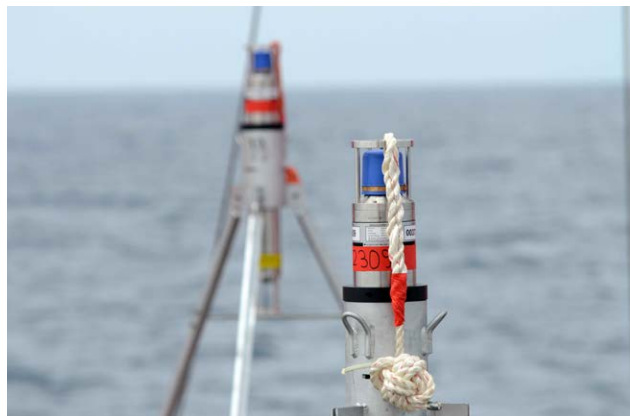
Figure 6.1.2.1: Autonomous Monitoring Transponder (AMT) installed in tripod frame (J. Steffen).
