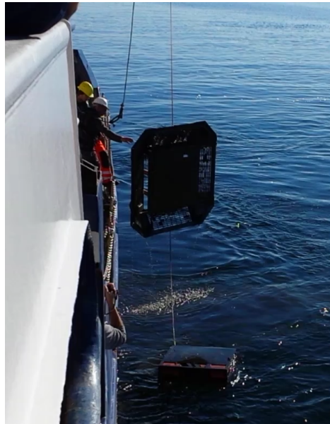
Figure 4.7: Recovery of the mooring. The buoyancy part had been triggered but could not float to the surface
