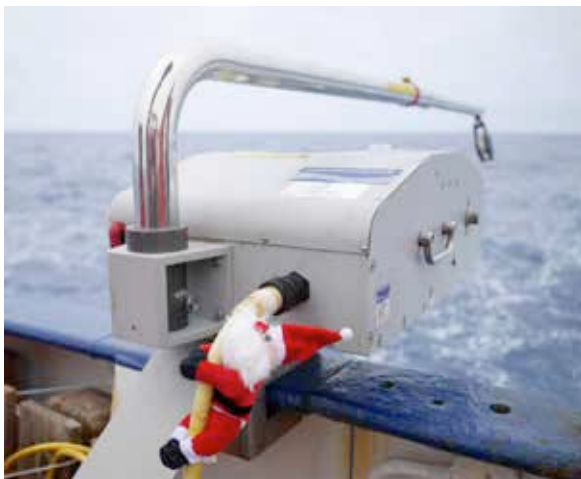
Winch of U-CTD at the stern of METEOR.
