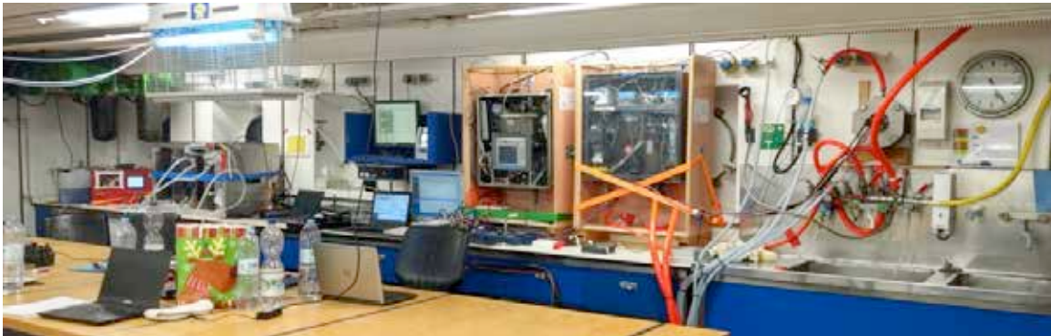
Systems to continuously observe the surface parameter such as carbon dioxide, oxygen and methane. Foto Tobias Hahn.
