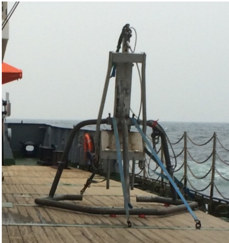
Figure 4: The employed giant box corer (box not installed) during the cruise POS489
