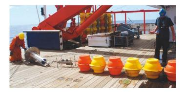
Figure 2: Moored instruments are prepared for deployment during a research cruise. Typical moorings in the oxygen minimum zone or near the equator contain an ADCP (white cylinder with transducers to the left), temperature, salinity and oxygen sensors (in the cage, middle-left), and buoyancy elements that hold the mooring upright in the water column (yellow and orange balls).
