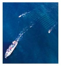
Figure 2: aerial view of a P-Cable system deployed from a research vessel. Photo: Geometrics Inc.
