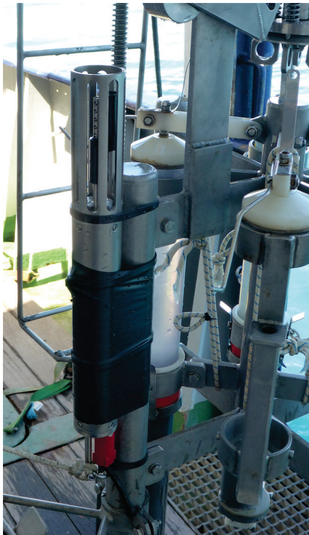
Fig. 12: Mini pushcorer (also short MIC) with CTD mounted (left) on board R/V Poseidon .
