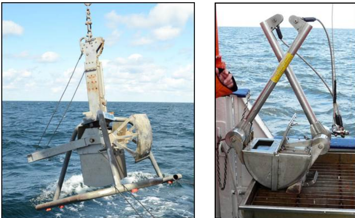
Figure 2: Giant grab sampler (GGS) (left) and Van-Veen-Grab-Sampler (right).
