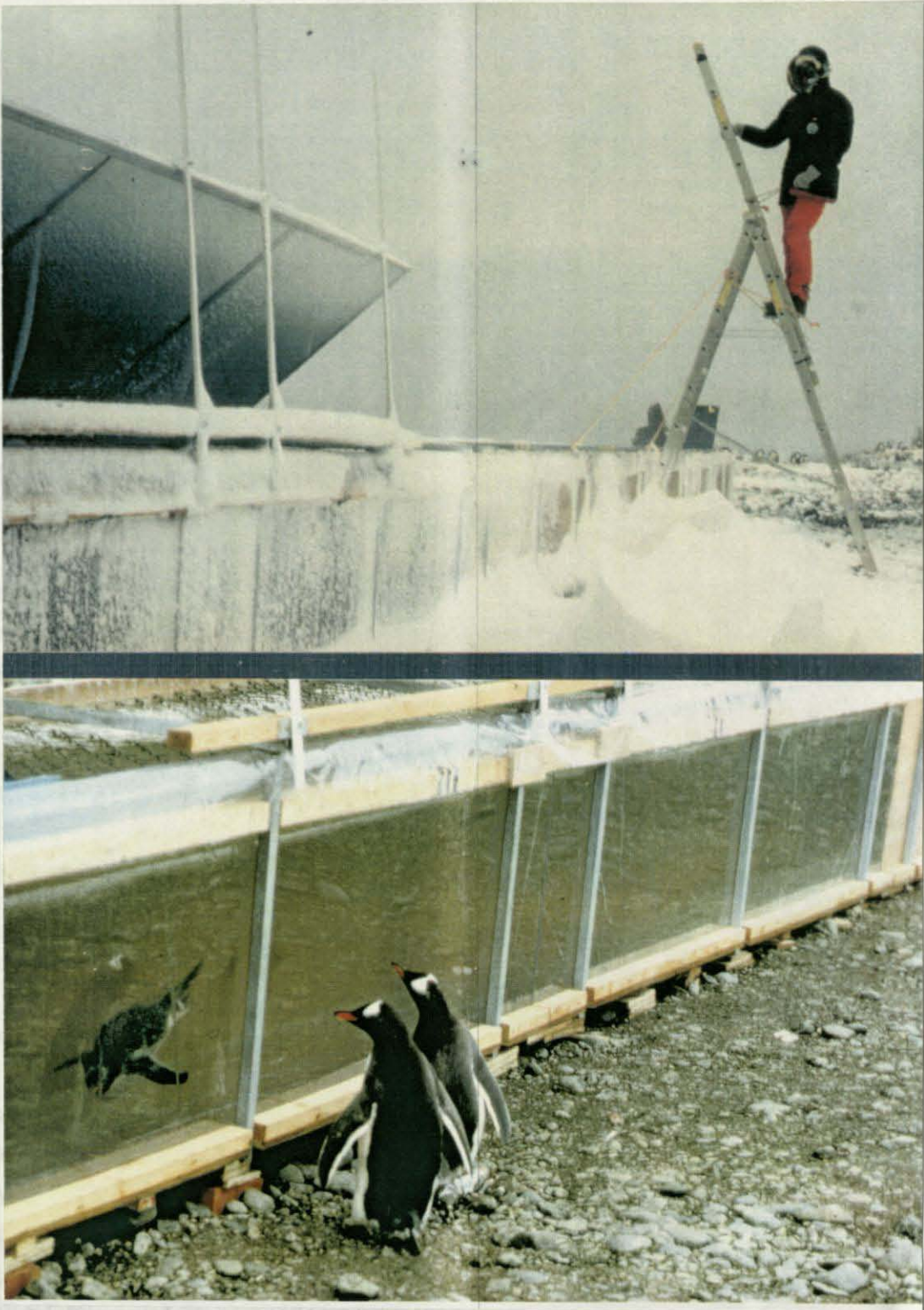
Fig 4: (Top) The swim canal was 21m long and covered with transparent PVC-glass sheets to prevent the penguins from surfacing. The birds could only obtain air in the respiration chambers placed at each end of the canal. Behaviour of the penguin in the canal, as well as swim speed and - distance were observed from above using a head-set microphone and a tape recorder. The mirror on the left was used in a project aimed at studying swimming kinematics. (Bottom) While swimming in the canal, this Gentoo penguin is being coached by two conspecifics awaiting their turn. The birds learned within a few minutes where they could surface to breathe and were generally very cooperative.
