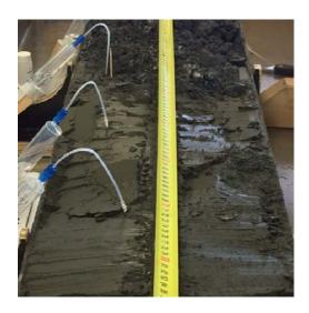
**Photo:** Pore fluid sampling in hydrothermally altered ("baked") mud from Kolumbo crater. Pore fluids are extracted using Rhizon samplers with 4- cm long porous membrane filters (0.12-0.18 micron pore size). Pore fluids were extracted within 1-2 hours after opening of each core.
