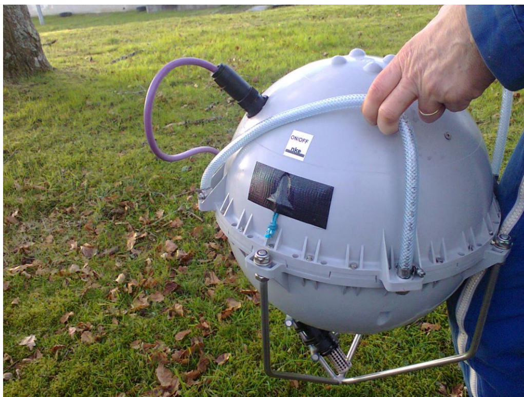
Figure 5: Picture of the demonstrator at EUMETNET/Météo-France premises, on 29 December 2016. Note the magnet to turn ON/OFF the buoy.
