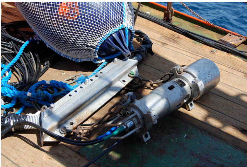
Figure 5.3.1.2: GI-gun mounted below the carrier to which a Polyform floatation is attached.
