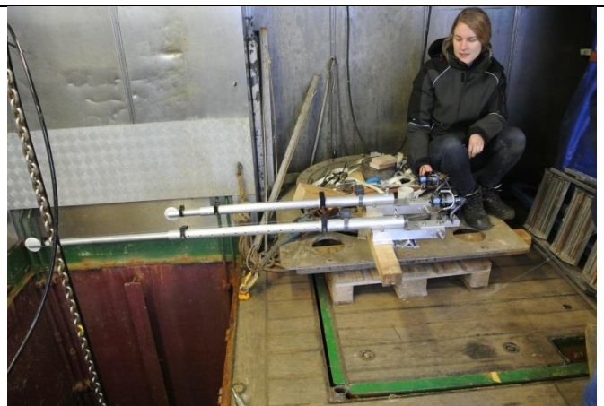
Figure 2: Setup during calibration of the EK80. The calibration sphere was deployed through the moon pool using four fishing rods to control its position below the sounder (in photo: Mareike Kampmeier). [Photo credit: Line Hähnel]
