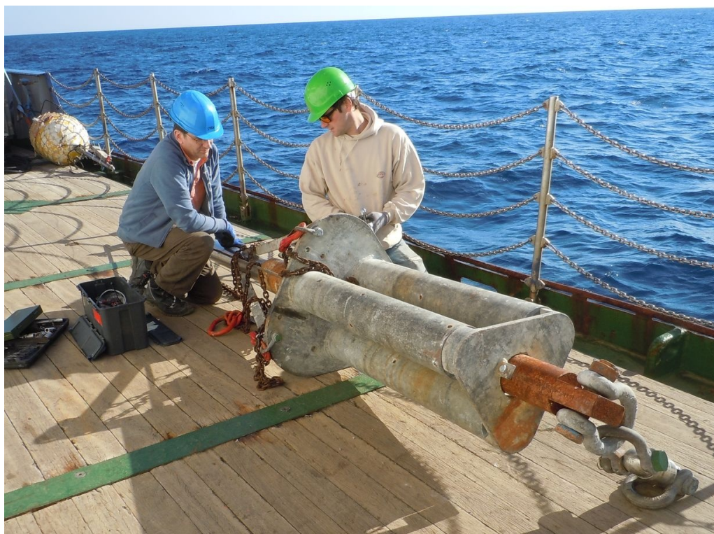
Fig. 16: Preparation of heatflow probe for deployment.
