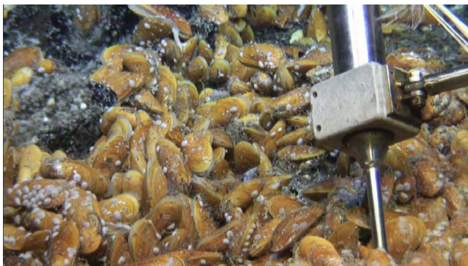
Fig. 2.4.3.4: Measurement of temperature with the 8-channel temperature logger at the low-temperature diffuse outlet at Wideawake (37 ROV13).
