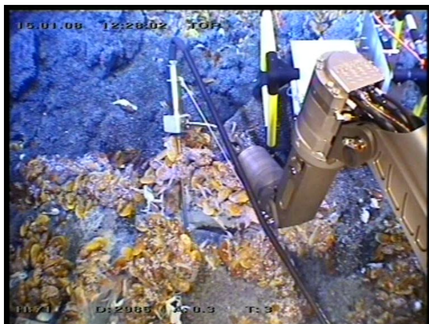
Fig. 2.4.3.2: Measurement of temperature with the 8-channel temperature logger at the low-temperature diffuse outlet at Wideawake (37 ROV6).
