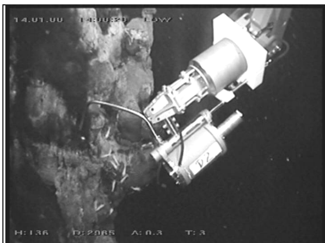
Fig. 2.4.5.3: Sampling of Two Boats with the Ti-Major sampler
