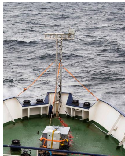
Bow of the Poseidon with the eddy covariance mast for the eddy covariance measurements. (Photo: Lisa Hoffmann)
