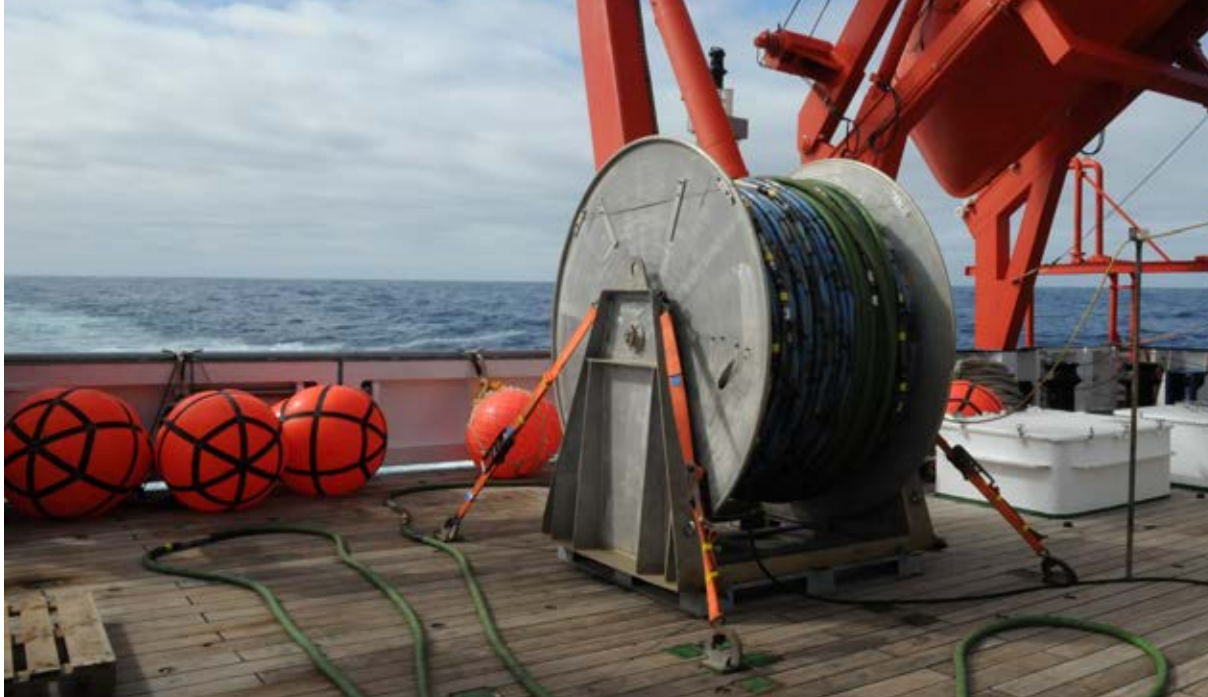
Figure 5.5: Streamer on winch on aft deck of RV Maria S Merian.
