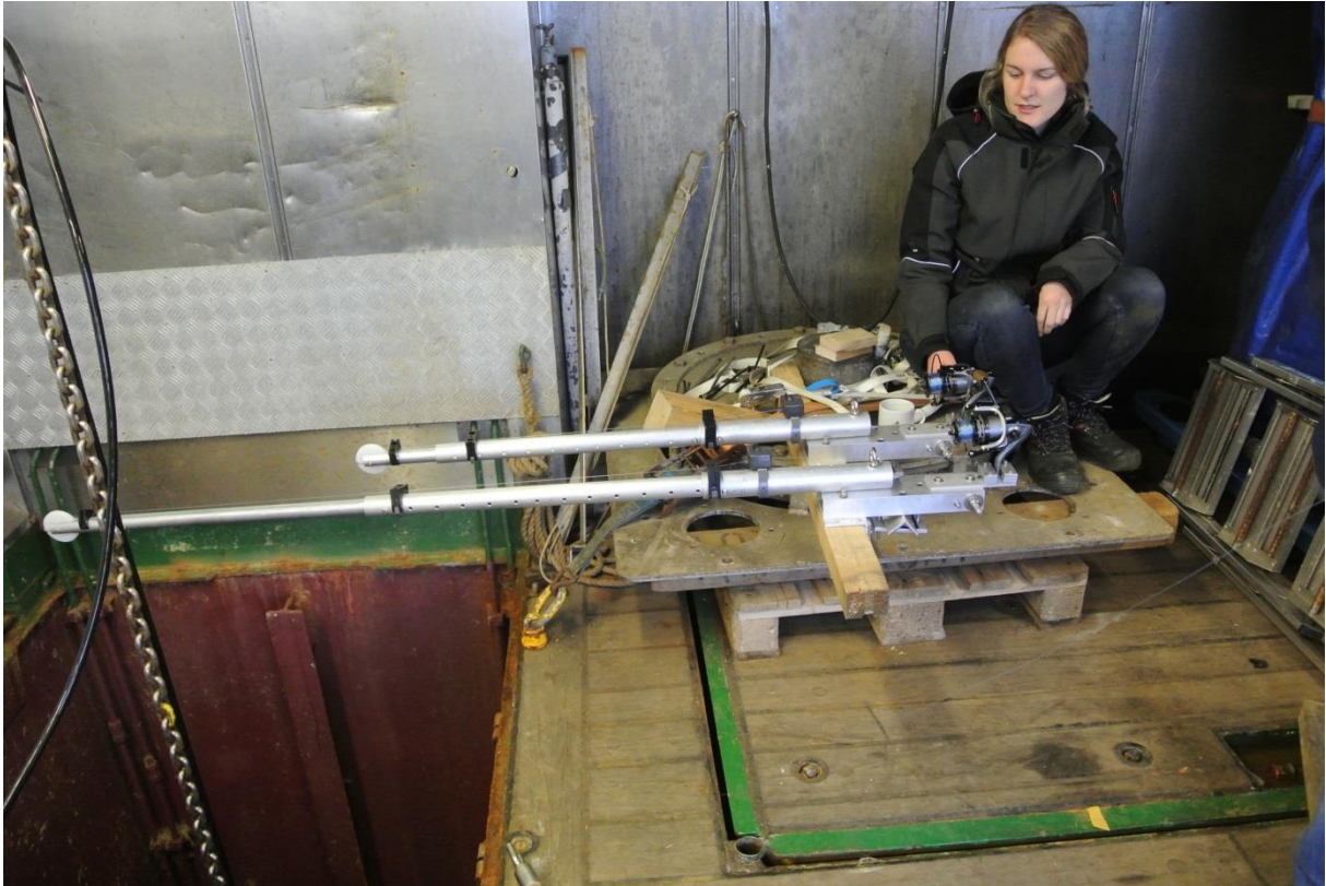
Figure 11: Calibration racks with fishing lines attached to the calibration sphere which is already below the moonpool. (Foto credit Line Hähnle; in picture: Mareike Kampmeier)
