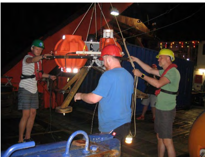
Fig. 1: Deployment of a bottom pressure sensor (photo: Martina Nielsen).
