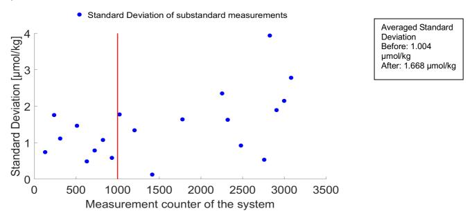
**Fig. 5:** Standard Deviation of substandard measurements in dependence of the measurement counter of the system. The red line denotes the time where the leakage started.
