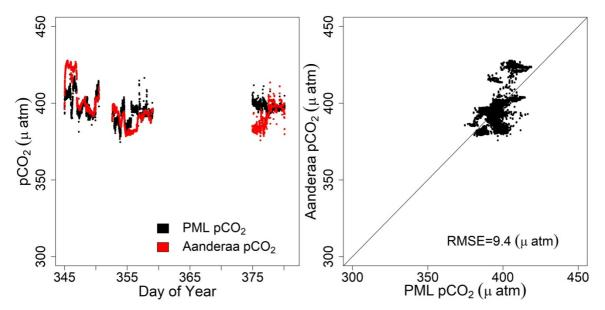
Figure 4:  $pCO_2$  as measured with a prototype optode sensor (Aanderaa  $pCO_2$ ) and established instrumentation (PML  $pCO_2$ ; Dartcom system) against time in 2015 (left panel).  $pCO_2$  from the optode sensor against the standard system (right panel; the solid line represents the 1:1 line).
