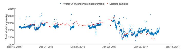
**Fig. 6:** Total alkalinity of the semi-continuous underway CONTROS HydroFIA® TA measurements and the discrete samples in dependence of the time.
