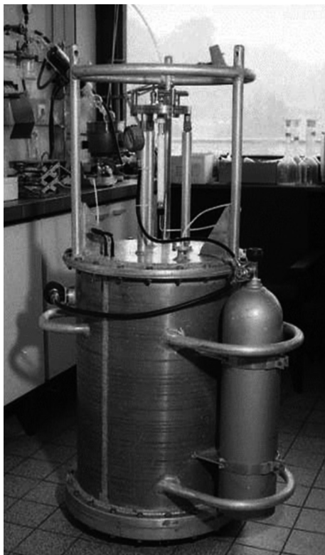
Fig. 25. Submersible version of the extraction buoy. Critical components of the machinery are pressurized with an aqualung. (Photo: M. Ehrhardt)
