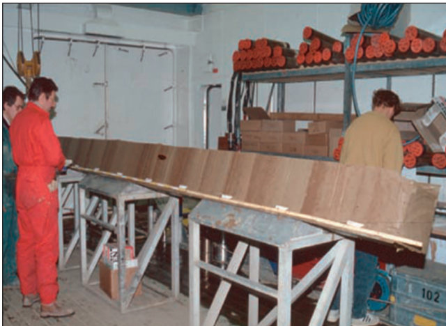
Fig. 6. “Kastenlot” from the central Arctic Ocean and acquired by research vessel POLARSTERN (long and large volume box corer developed by the marine geology group of GPI).
