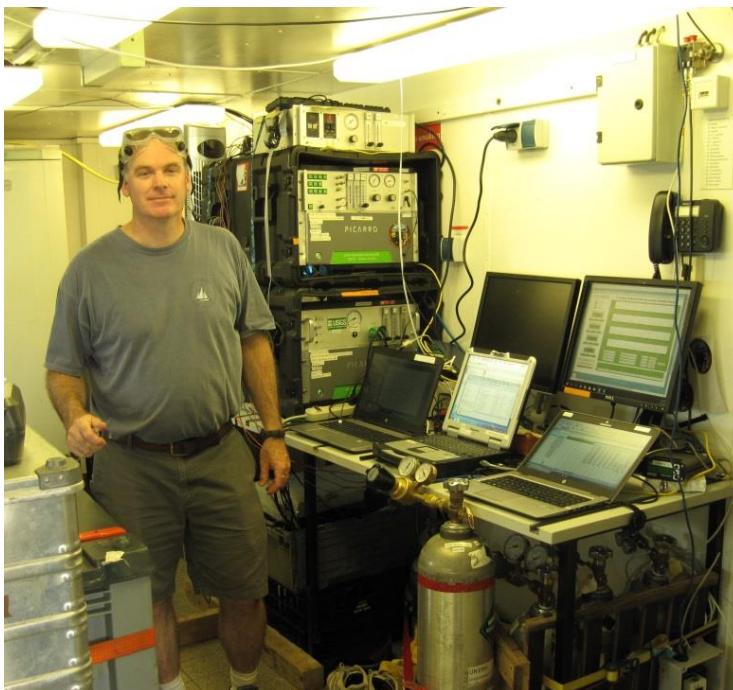
The USGS GAS - CRDS system with Michael Casso running direct injections. Michael was the main person analysing 277 samples for CH 4 , CO 2 AND its \delta^{13}C ratios (not including the standards).
