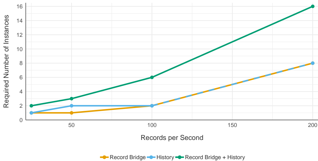
Figure 7.6. Lowest number of instances that is able to process a certain number of measurement records per seconds.
