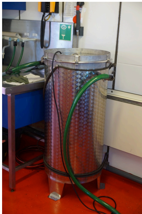
Fig. 5.11 Stainless steel barrel for passive sampling of organic pollutants dissolved in seawater
