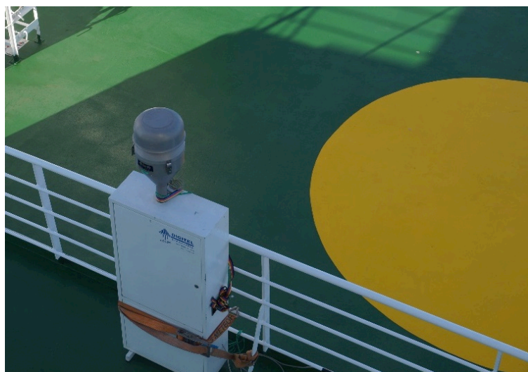
Fig. 5.12 Digital High Volume Sampler (view from bridge)
