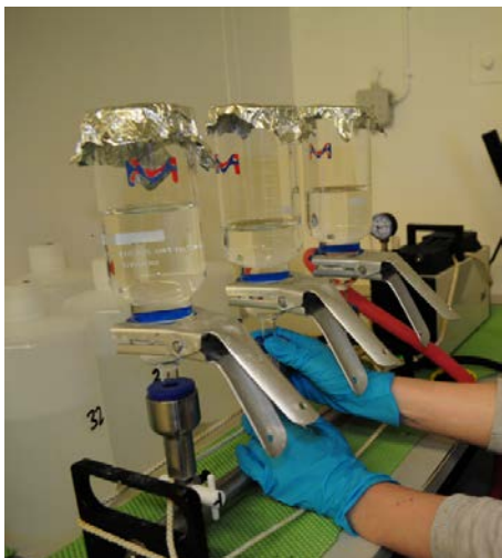
Figure 3: The filter set up for eDNA sampling showing water inside the glass beakers, the manifold which holds the beakers and the pump which sucks water through the filters.
