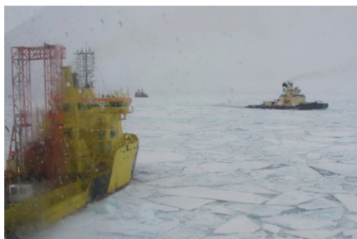
Fig. 1: Drilling platform "Vidar Viking" in the foreground. Swedish icebreaker "Oden" and Russian icebreaker "Sovetskiy Soyuz" in the background smashed the drifting sea ice in order to keep the position of the drilling platform stable.
