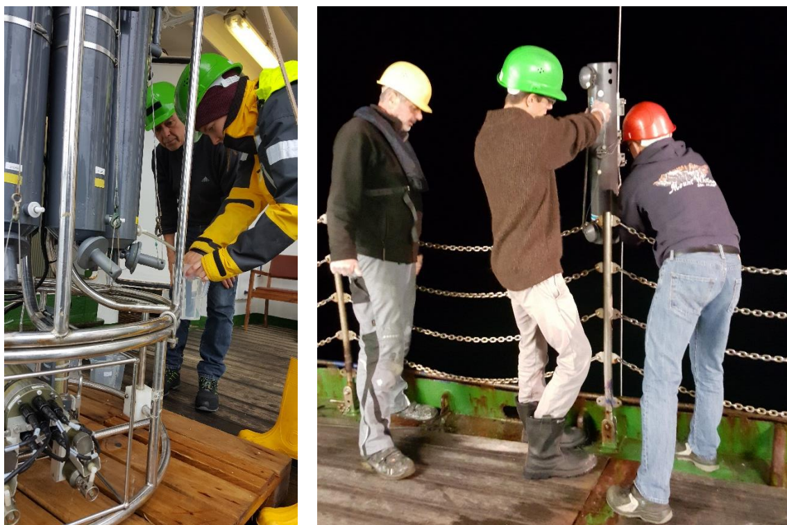
Figure 9: (Left) Collecting water from the CTD bottles for explosive analysis. (Right) Deploying GoFlo bottles for trace element sampling.
