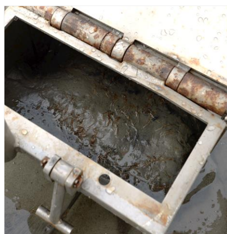
Figure 2: Using a VanVeen – grab to get seafloor samples. The sediment is sampled for grain size and porosity analysis, such as for chemical studies.
