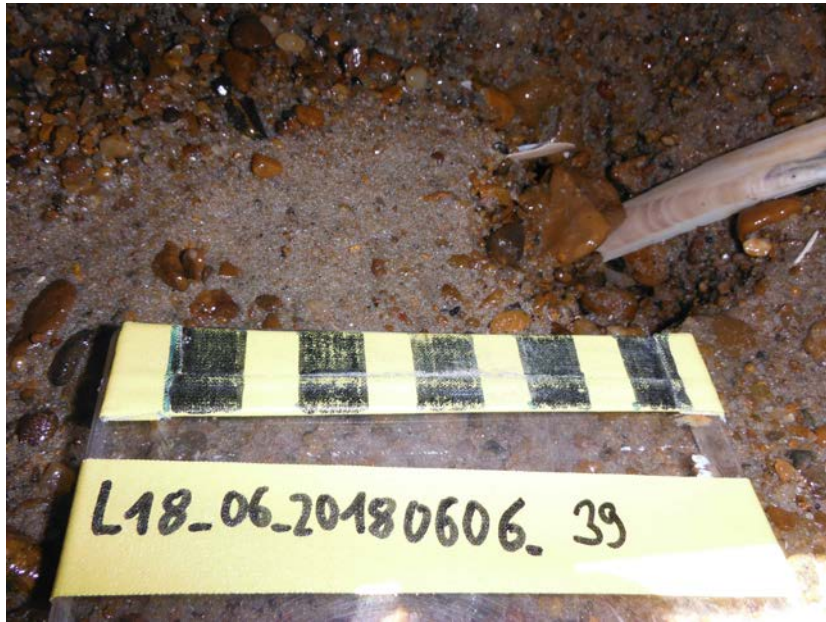
Figure 5: Photo of grab-sample with coarse material.
