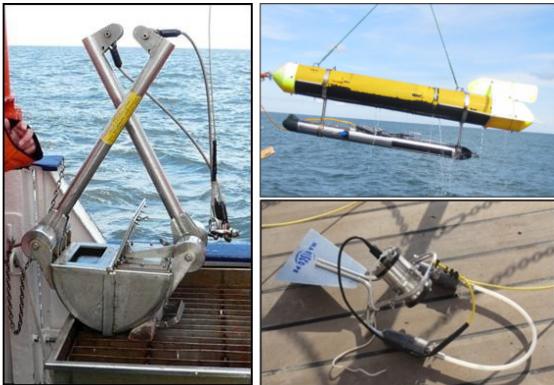
Figure 2: Van-Veen-Grab-Sampler (left), sidescan sonar and underwater video system (right).
