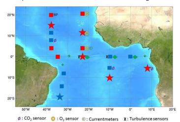
The present PIRATA network: the meteo-oceanic buoys are represented by rectangles and by stars for Full Flux ones. T-Flex are colored in red and ATLAS in blue. ADCP moorings are represented by green diamonds. Additional symbols are explained in the map legend. All meteo-oceanic buoys are equipped with OTN. Green crosses represent islands where some tide gauges and meteorological stations are/were also maintained.
