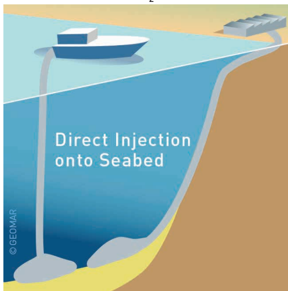
Figure 5.6 Liquid CO 2 placed on the seabed
