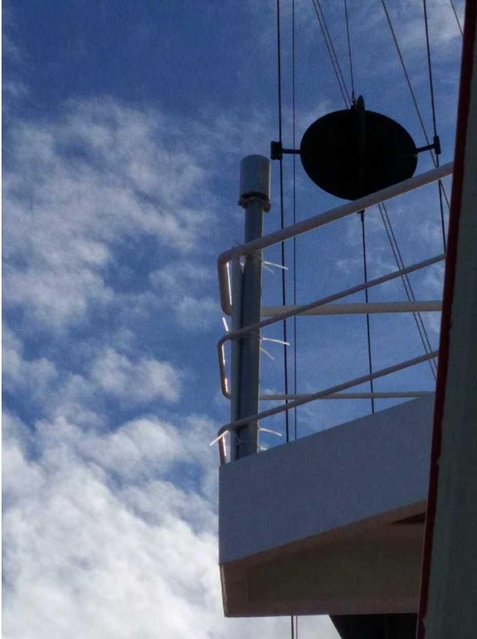
Fig. A3.2 Fluxgate magnetometer installed above the observation room of RV Sonne, starboard side.
