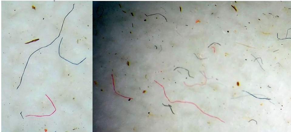
Fig. 5.12: Photography of plastic fibers from surface waters off Peru on a GFF filter.
